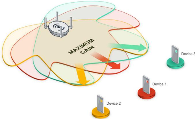
FIGURE 4: MU-MIMO DIRECTIONAL TRANSMISSION
