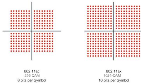
Figure 4: A comparison of constellation charts between 256-QAM and 1024-QAM modulation density.
