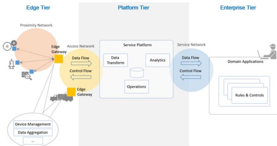
Figure 5: Three-tier IIoT system architecture.
