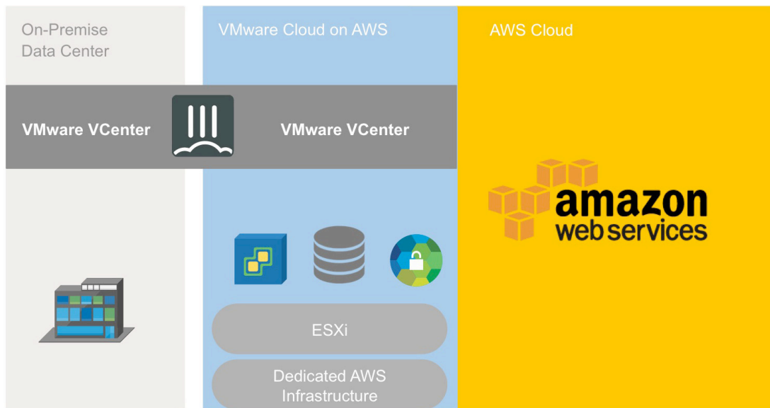
FIGURE 1: VMWARE CLOUD ON AWS ACCESS FLOW
