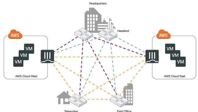
Figure 4: Enterprise distributed remote locations to create tunnels. Connecting AWS hosts to reduce bottlenecks.
