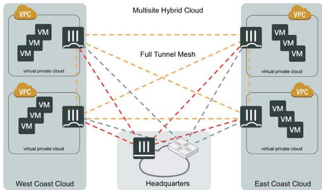
Figure 3: Full tunnel mesh connecting all VPCs with headquarters.
