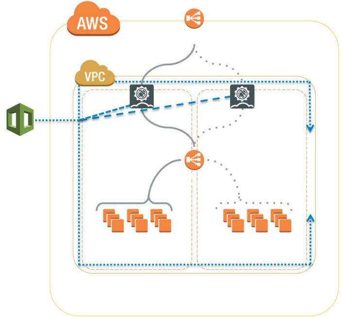
Figure 2: FortiWeb using Amazon ELB (In this case, we show an ELB Sandwich).
