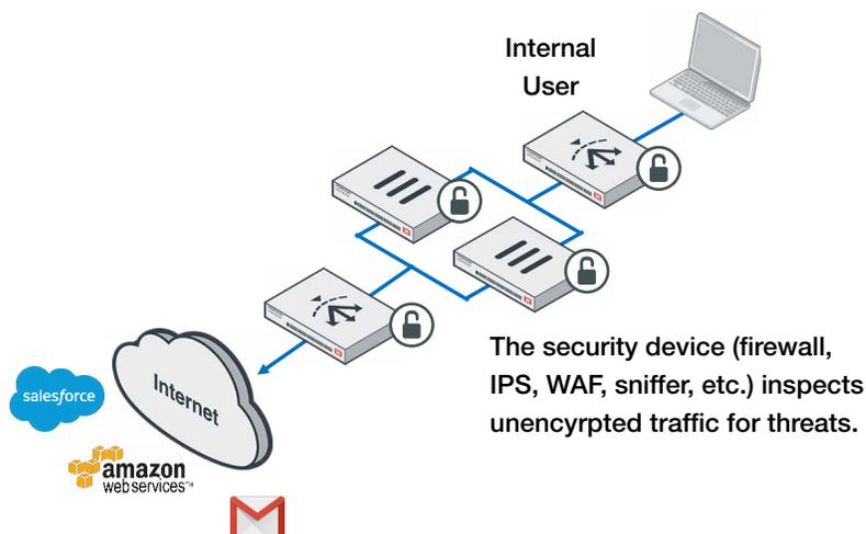
Figure 2: FortiADCs provide encryption and decryption services and can load balance multiple firewalls or other security devices.
