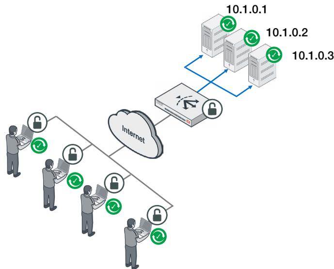
Figure 1: FortiADCs decrypt and encrypt traffic to/from users, allowing servers to focus on load-balancing applications to improve application performance.
