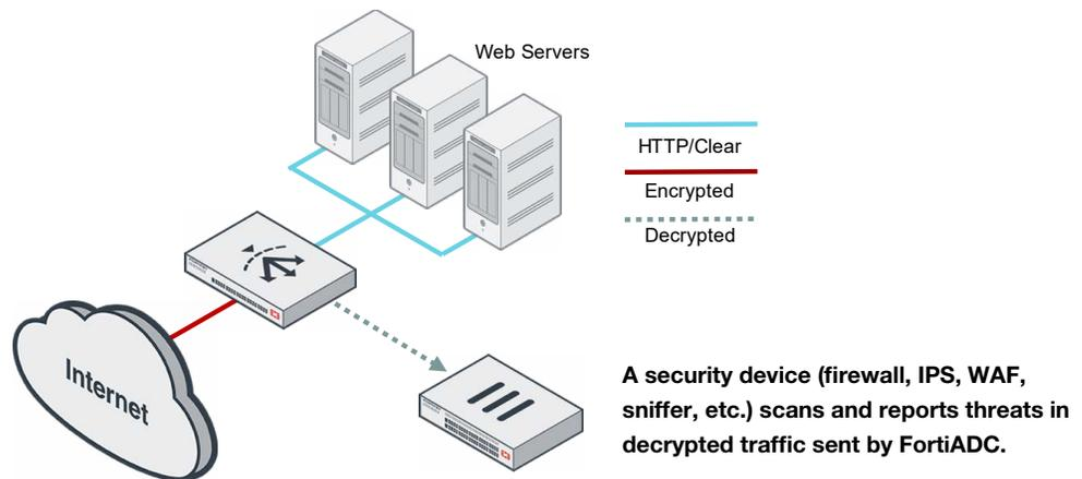
Figure 3: FortiADCs load balance traffic to servers, offload SSL traffic, and send mirror copy of decrypted traffic to the security device.
