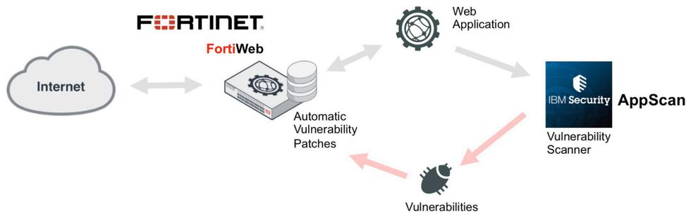
IBM Security AppScan scan results are imported into FortiWeb; then FortiWeb Virtual Patching automatically creates new rules to protect against newly discovered vulnerabilities.
