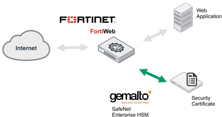
FORTIWEB CAN BE CONFIGURED TO USE SSL/TLS CERTIFICATES AND ENCRYPTION KEYS STORED AND MANAGED BY THE SAFENET ENTERPRISE HSM.
