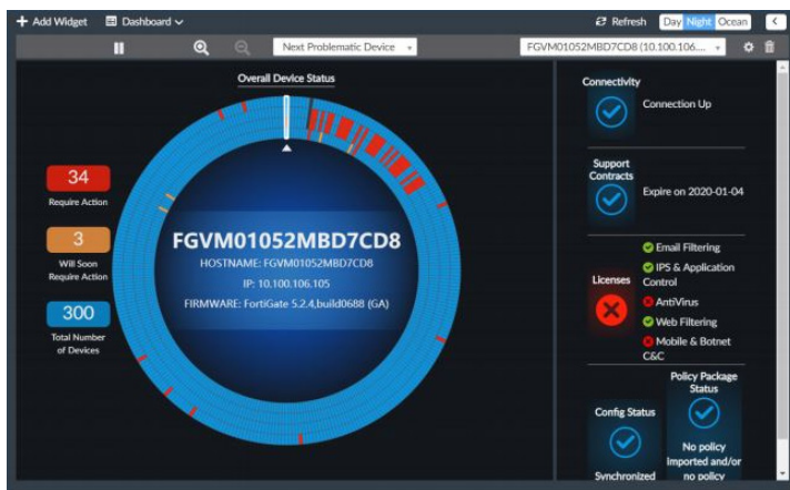
Figure 2: NOC-SOC Device Status Dashboard
