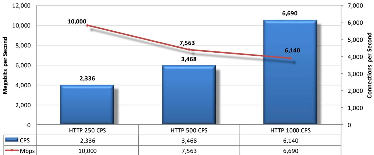
Figure 13 – HTTP Capacity HTTP Persistent Connections
