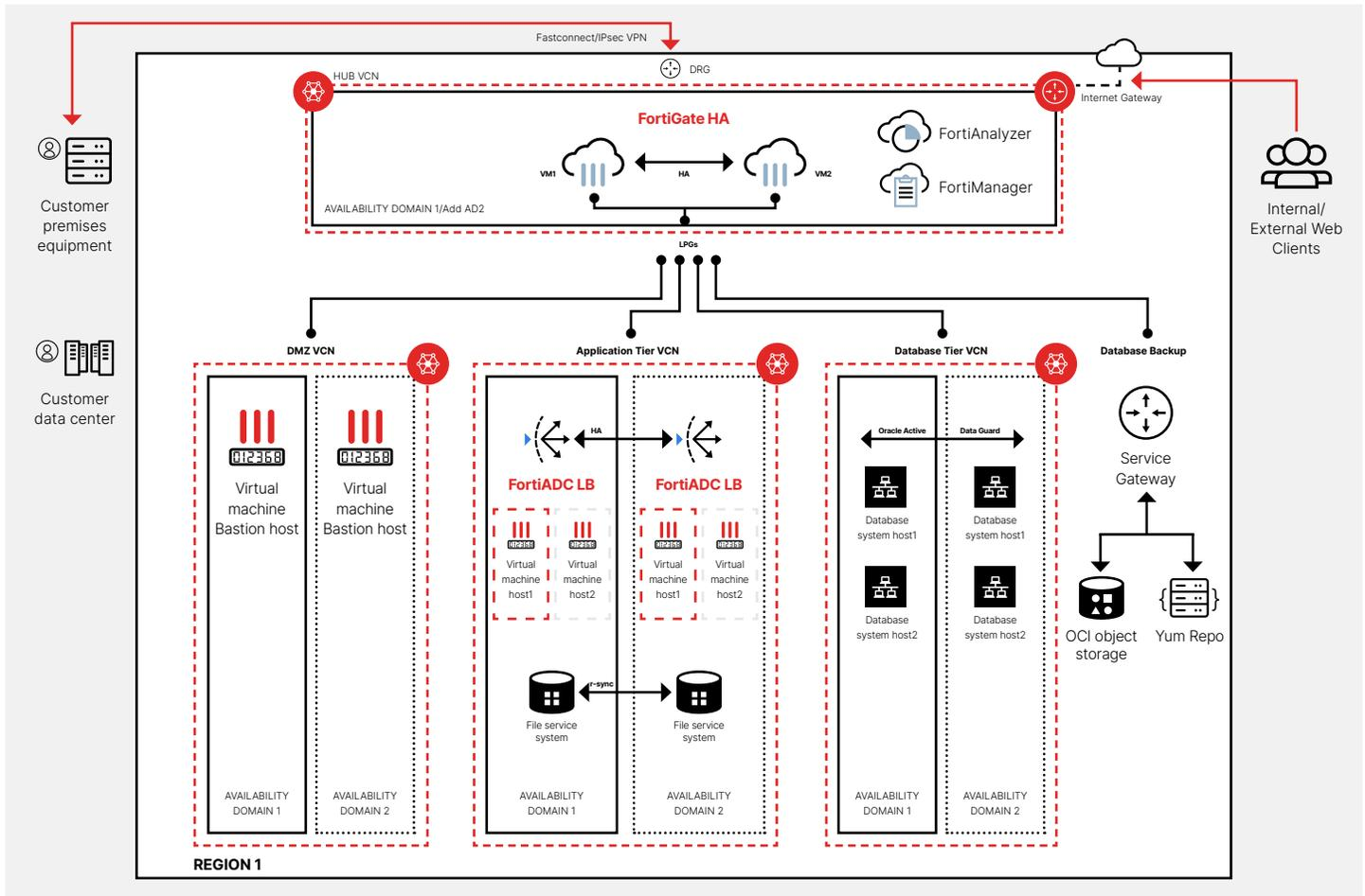
Figure 3: Oracle EBS and Fortinet security solution blueprint.
