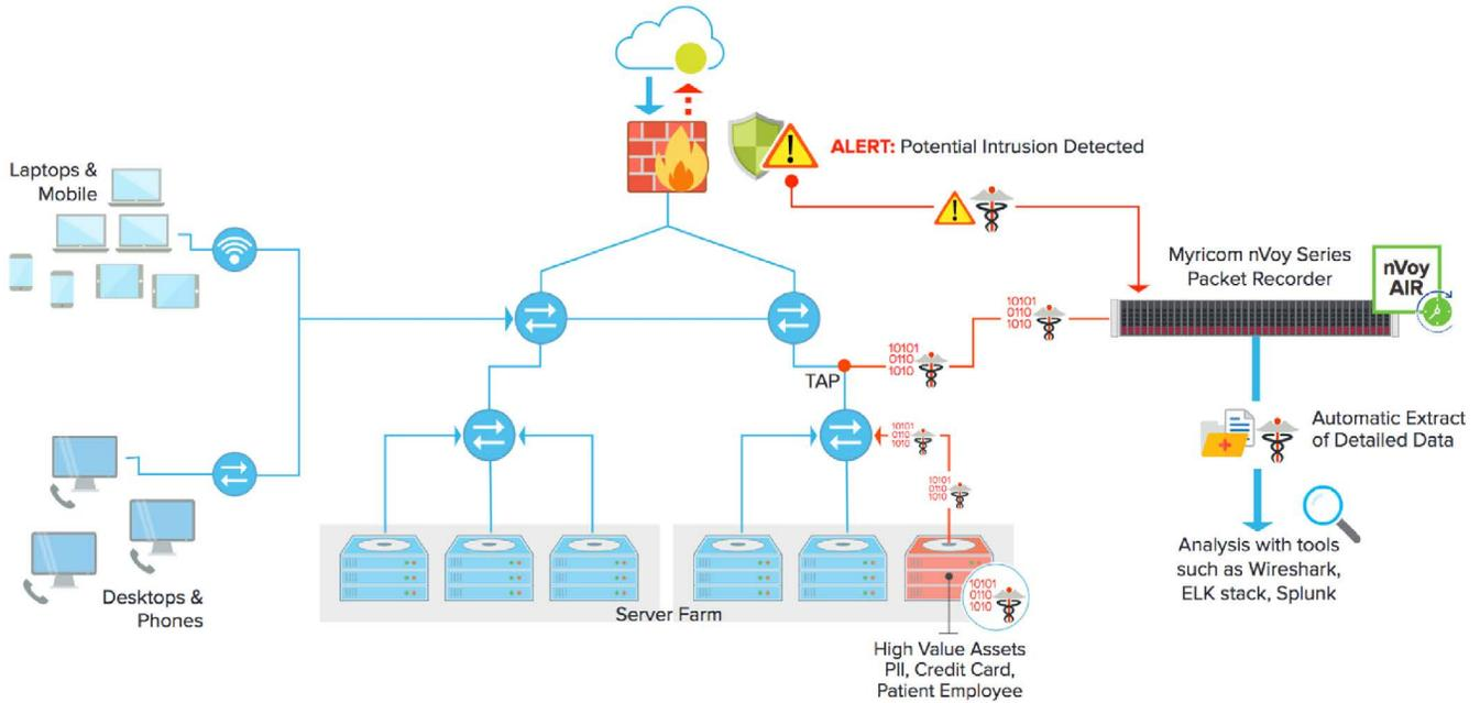
Figure 1: Myricom nVoy air watching critical assets and ready to respond to intrusion events.
