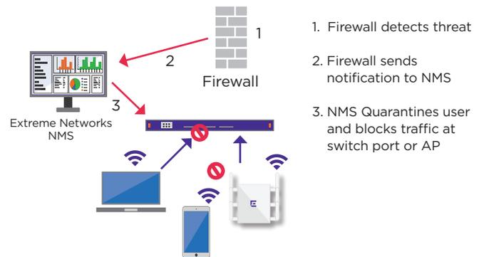
Figure 4. Enforcement at Switch Port or AP
