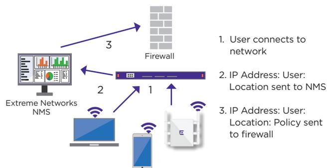
Figure 1. User to IP Address Mapping
