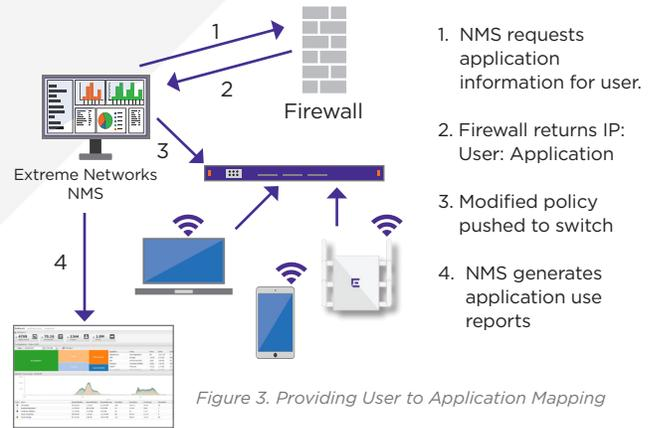
Figure 3. Providing User to Application Mapping
